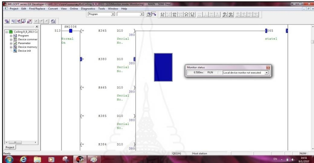
Figure 27: Ladder diagram shows Y65 operate
