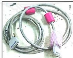
Figure 4: Cable GT15-QC30B link between PLC and Touchscreen
