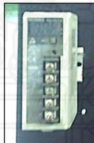
Figure 7: Power supply 24VDC
