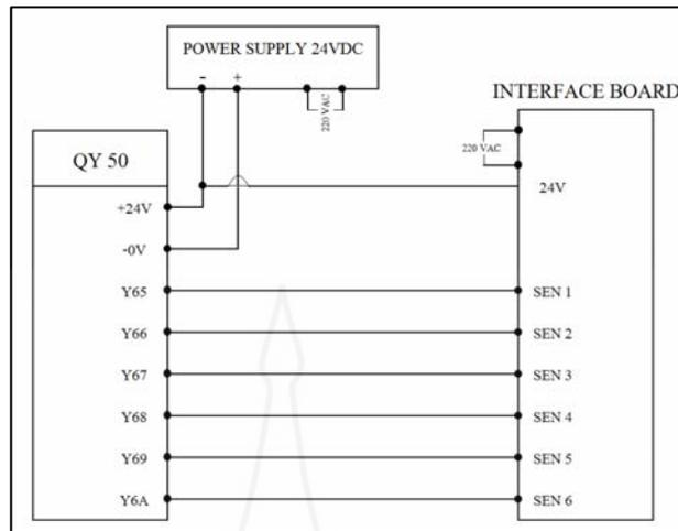
Figure 17: Wiring diagram for test device
